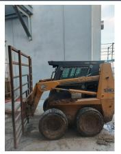
A skid steer with a gate welded on the front
